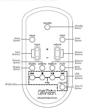
Standby button: press this button to put the unit into and out of the selected Standby mode.
